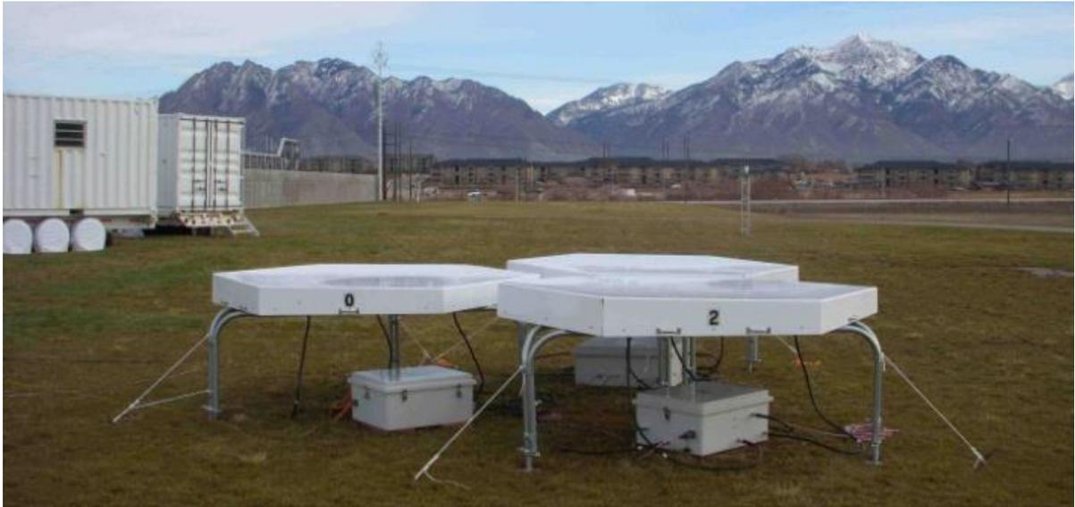
**Figure 1:** Prototype 3-antenna 449 MHz wind profiler Salt Lake City, UT for PCAPS, Nov 2010.
