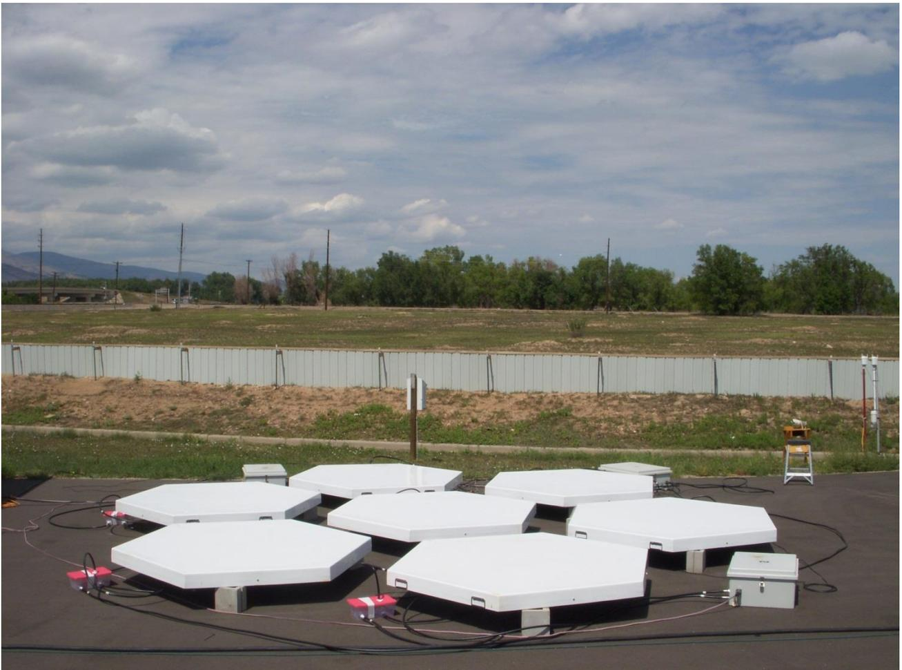
**Figure 3:** Prototype 7 antenna module 449-MHz wind profiler, under construction.
