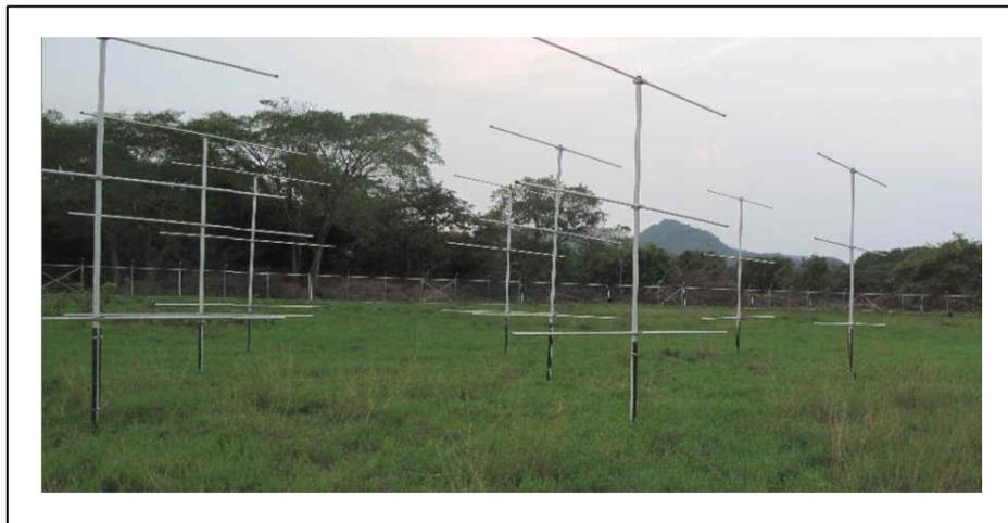
**Figure 3:** Transmitter array used in the experiment.
