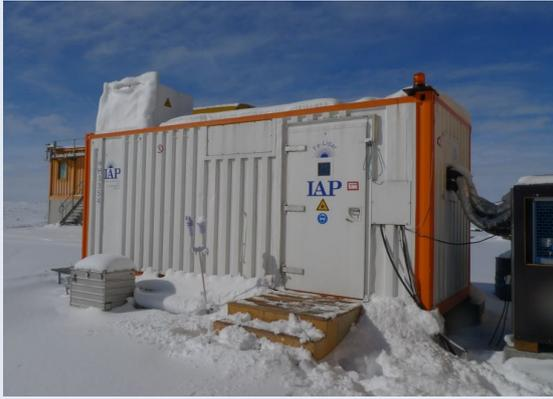
**Figure 7:** The mobile IAP Fe lidar at Davis, Antarctica (69°S) in March 2011. The system is housed in a single insulated 20' container, designed to be transported to remote polar regions. CC BY-NC 4.0
