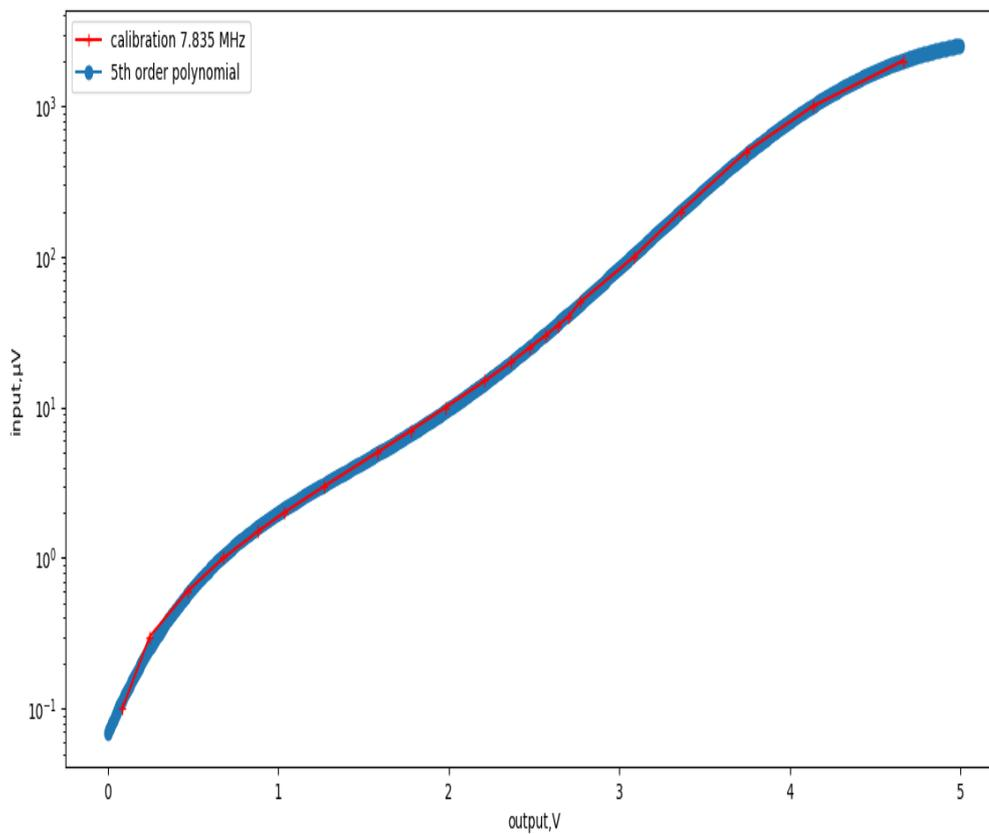
Figure 3.10: Polyfit function with Over fitting (non - generic).
