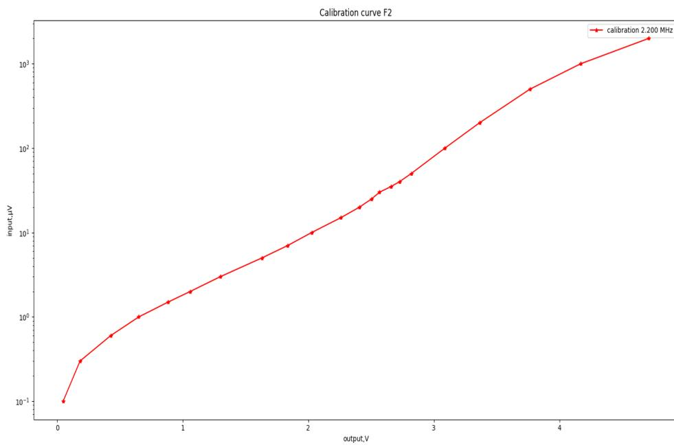
Figure A.15: Calibration Curve (V vs.  $\mu\text{V}$ ) for frequency 2 = 2.200 MHz
