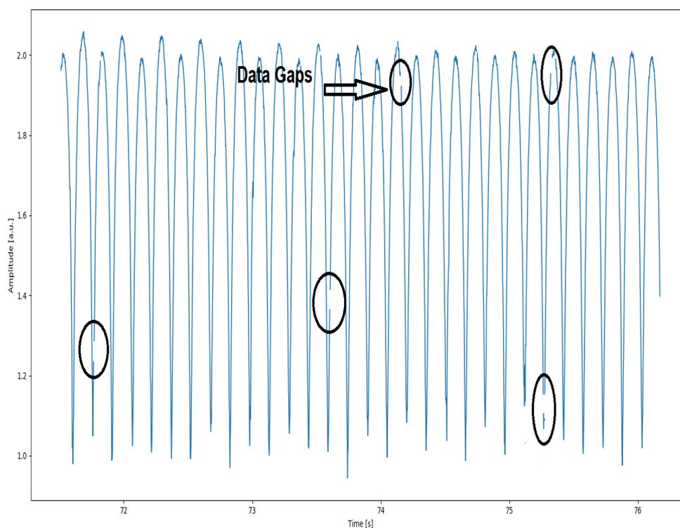
Figure 3.6: Data from 72 to 76 (sec) of Frequency 4 = 7.835 MHz without interpolation with large data gaps.
