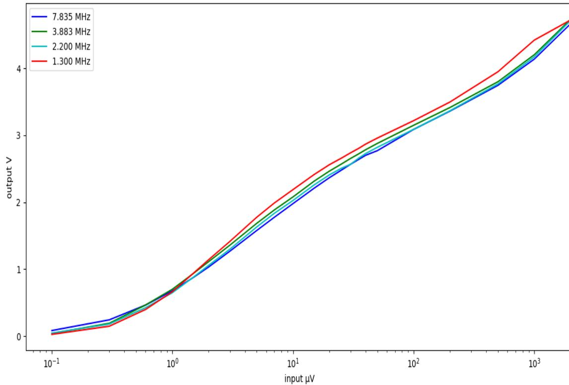
Figure 3.4: Calibration Curve with all the frequencies ( $\mu\text{V}$  vs.  $\text{V}$ )
