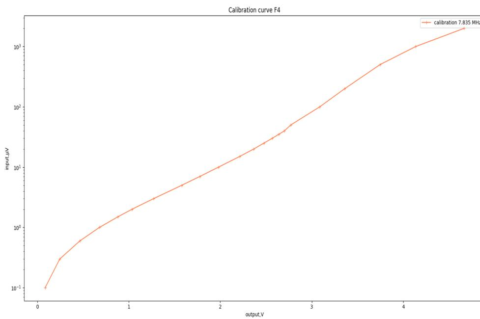
Figure A.13: Calibration Curve (V vs.  $\mu\text{V}$ ) for frequency 4 = 7.835 MHz
