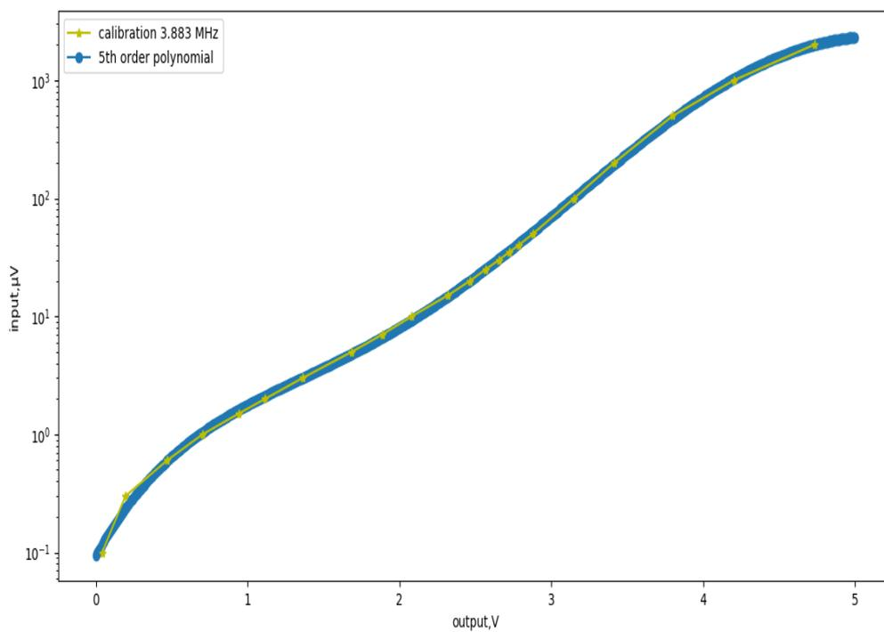
Figure A.17: Calibration data: Polyfit function of frequency3 = 3.883 MHz (5th order)
