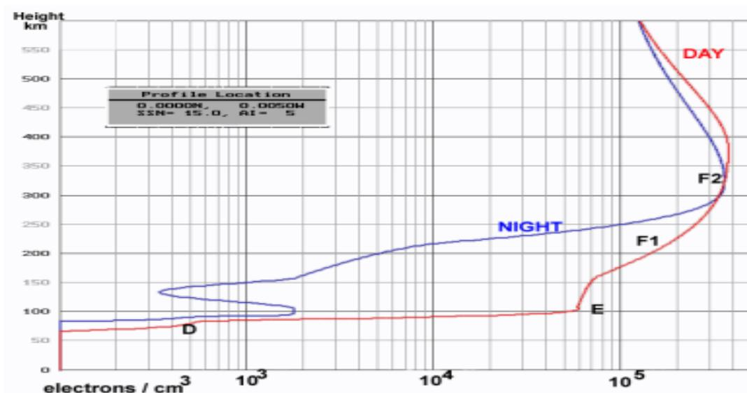
Figure 1.3: Ionospheric Layers during Night and Day.([1])
