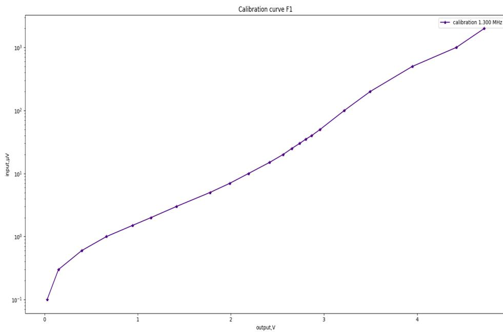
Figure A.16: Calibration Curve (V vs.  $\mu\text{V}$ ) for frequency 1 = 1.300 MHz
