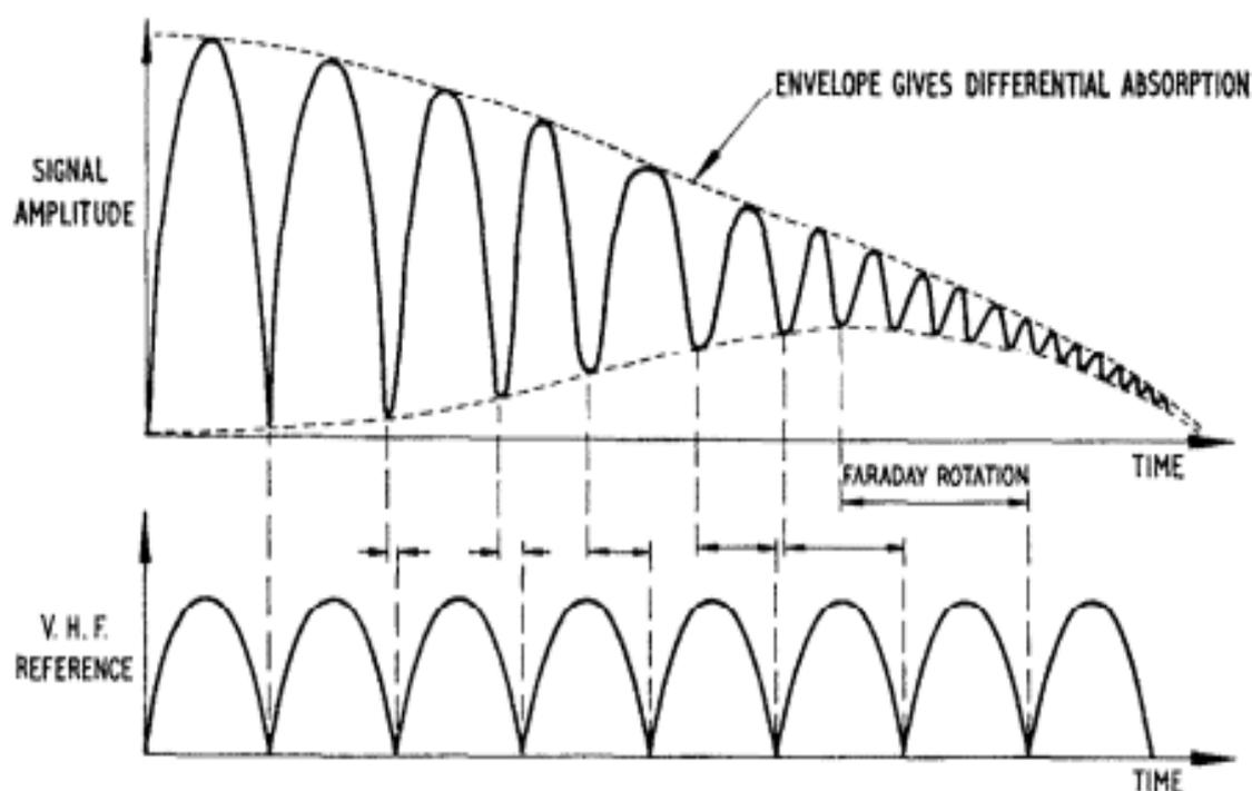
Figure 2.5: received rocket signal emphasize the measurement of Faraday rotation and Differential absorption. ([7])
