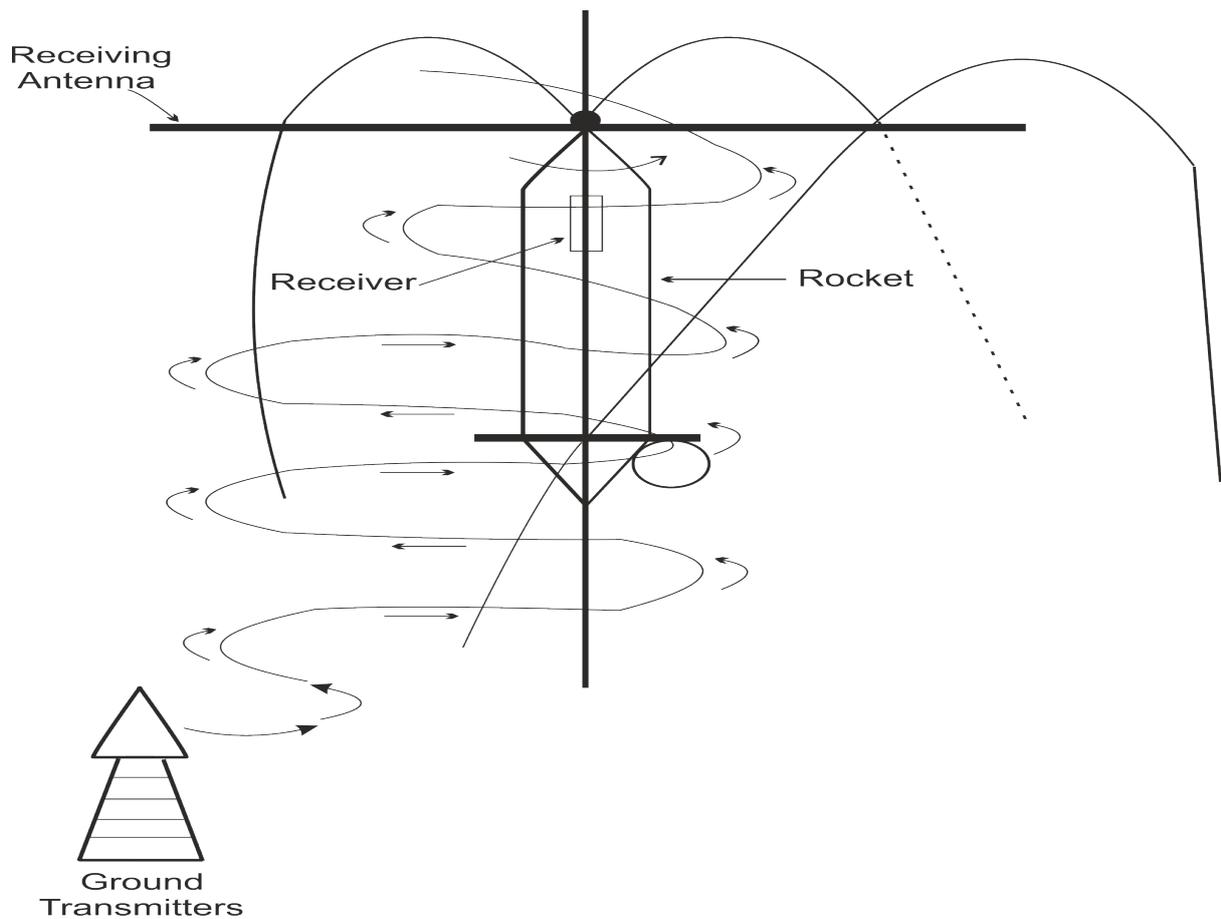
Figure 3.1: Experiment description with the receiving antennas on the board of the sounding rocket.
