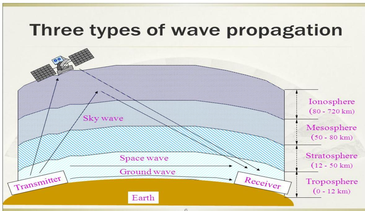
Figure 2.2: Types of Wave Propagation.([1])
