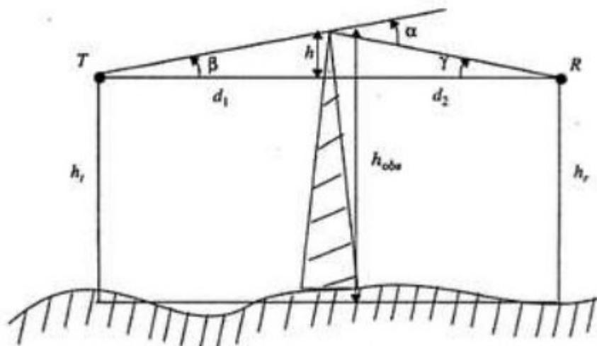
Figure 2.3: Knife-edge diffraction geometry. The point T denotes the transmitter and R denotes the receiver, with an infinite knife-edge obstruction blocking the line-of-sight path. [[2]])
