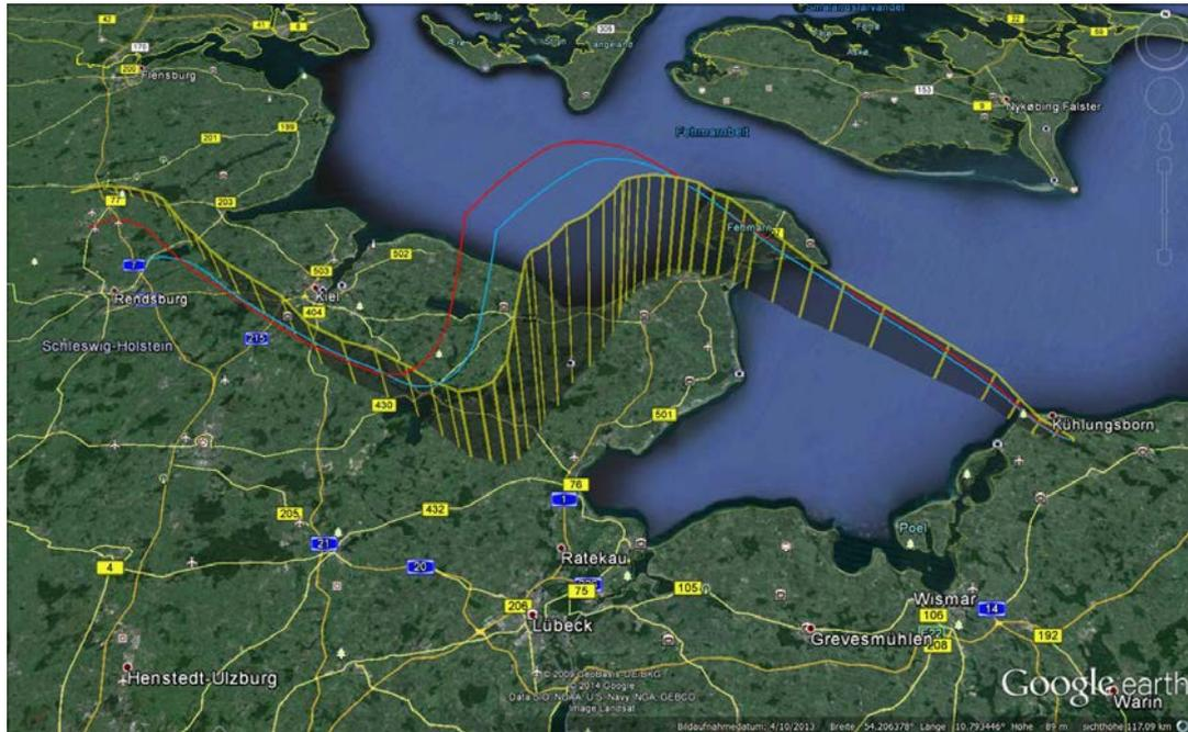
Figure 3.21.: Flight track predictions for 27<sup>th</sup> March 2014. The blue line is the last forecast that was available prior to launch, the red one uses the 06:00 run of GFS-model which could be accessed only after take off, whereas the yellow one shows the true flight path of LITOS.
