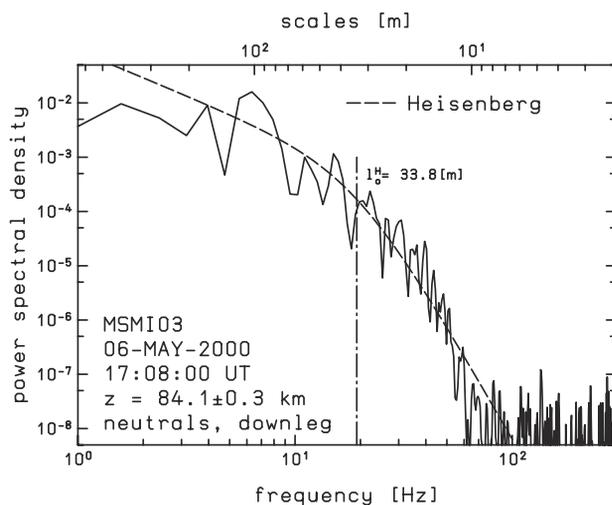
**Figure 3.** Power spectral densities of the relative density fluctuations versus frequency (lower axis) and scale (upper axis) from flight MSMI03 at an altitude of  $84.1 \pm 0.3$  km. A Heisenberg spectrum of turbulence calculated from the best fit results (see text) is shown by the dashed line.  $l_0^H$  denotes the inner scale of the Heisenberg model.
