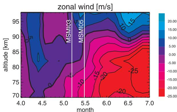
**Figure 1.** Background zonal winds from the MF radar at altitudes from 70 km to 98 km in April, May, and June 2000. The contour colors range from blue = eastward (positive values) to red = westward (negative values) winds. The contour level of 0 m/s is emphasized by a thick black line. The times of the MIDAS launches are marked by white vertical lines.
