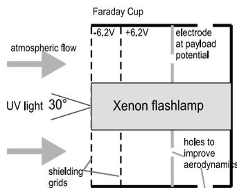
**Figure 1.** Schematic of the particle detector.
