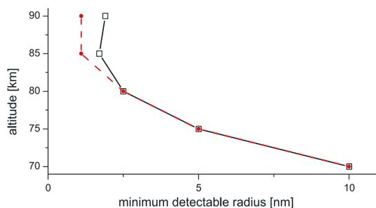
**Figure 2.** Minimum detectable radius of negatively (red line) and positively (black line) charged particles as a function of altitude.
