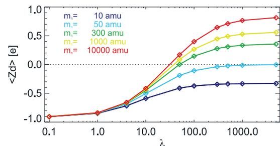
**Figure 5.** Mean particle charge (particle radius = 2 nm) as a function of the parameter  $\lambda = n_n/n_e$  for different assumed negative ion masses  $m_n$ .
