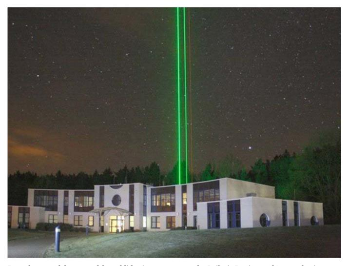
Laser beams of the ground-based lidar instruments at the Leibniz Institute of Atmospheric Physics in Kühlungsborn, Germany, slice through to an altitude of about 120 kilometers, collecting data in atmospheric regions along the way. Credit: © IAP, Kühlungsborn
