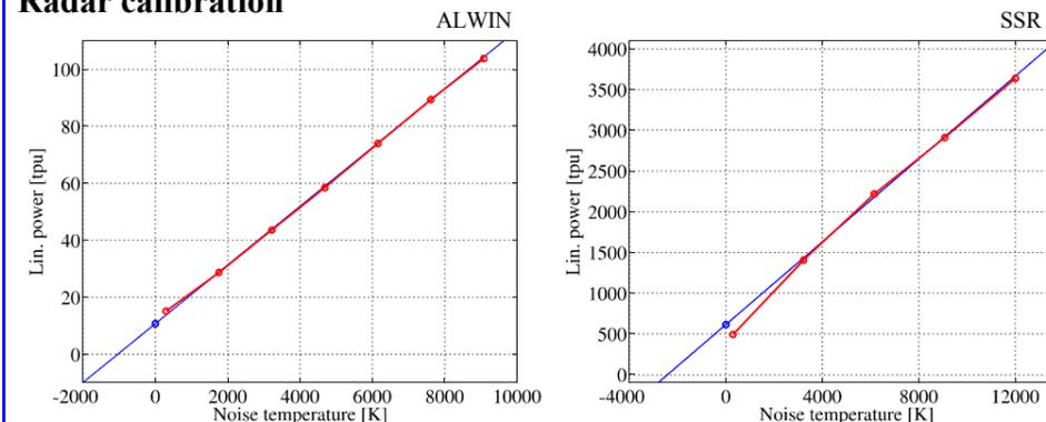
The pictures show output power  $P_{out-a}$  vs. noise temperature (red curve) after calibration measurements at ALWIN radar (left) and Svalbard SOUSY radar (right). A straight (blue) line  $P_{out-a} [tpu] = a + b T$  was fit into the curves with the parameters  $b = \Delta P_{out-a} / \Delta T$  and  $a = P_{out-a}(T=0)$  (blue dots). Since the input noise power is  $P_{inp-a} [W] = \Delta f k T = c T$  the calibration factor for incoherent signals can be determined by:
