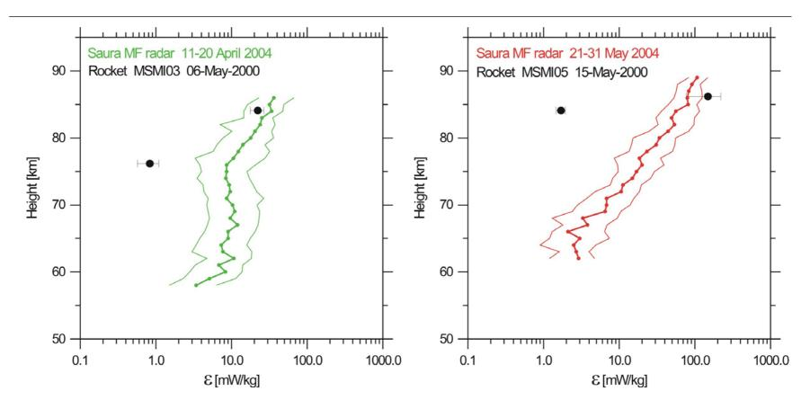
Mean ε profiles (medians & quartiles) before and after spring time wind reversal in 2004 compared with rocket soundings at comparable conditions in 2000.
