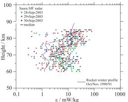
**Short time variability of \epsilon:** Hourly mean values (dots) of energy dissipation rates from three days radar observations in September 2003. The median (black line) derived from the spectral width measurements and the  $\epsilon$  profile (dashed blue line) from previous rocket soundings during winter are in qualitative agreement.
