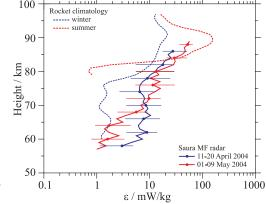
$\epsilon$  variations related to the spring transition of the mesospheric circulation:  $\epsilon$  profiles from radar (solid lines) and rocket measurements (dashed lines) before (blue lines) and after (red lines) spring transition of the mesospheric circulation in 2004. The horizontal bars indicate the range between lower and upper quartile.
