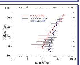
Summer to winter transition of turbulence: The  $\epsilon$  profiles based on radar measurements (mean values with standard deviation) show smaller values below 85 km in August (red) than in September/October (blue and black) but the inverse relation above 80 km. This relation corresponds qualitatively to previous rocket observations.
