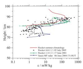
Individual profiles of turbulent energy dissipation rates: Individual  $\epsilon$  profiles derived from radar observations and rocket soundings are compared with a summer climatology based on sounding rocket data. The radar  $\epsilon$  profile shows also a steep increase of energy dissipation above  $80\,\mathrm{km}$  comparable to the in-situ data.
