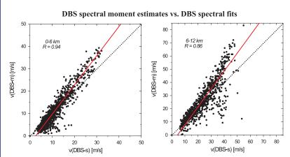
The wind magnitude determined by the three methods is in good agreement for wind speeds lower than about 20 m/s at altitudes below 6 km and lower than about 25-30 m/s at altitudes between 6 and 12 km.
